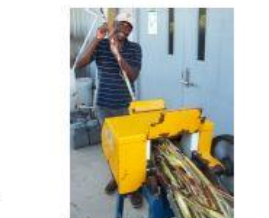
Figure 3: Juice extraction from Sweet Sorghum stems.
