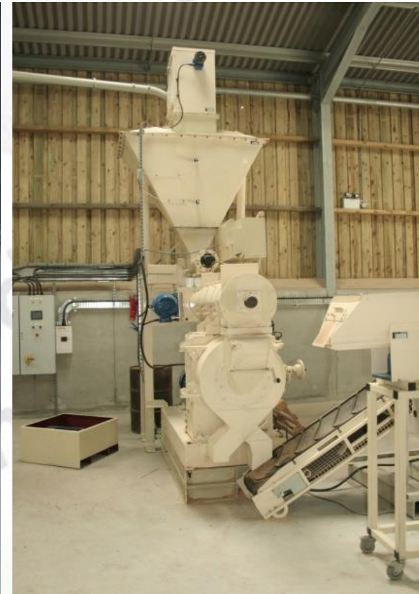
Dry processing: Pellet mill
